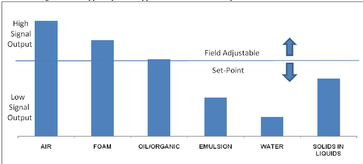
The field adjustable set-point can easily be set to detect interfaces between products with different thermal conductivities.
