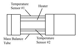
Temperature Differential = Temperature Sensor #1 Minus Temperature Sensor #2
