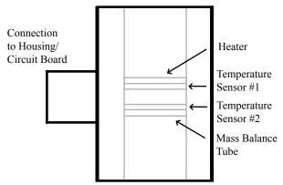
Temperature Differential = Temperature Sensor #1 Minus Temperature Sensor #2
