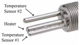
Temperature Differential = Temperature Sensor #1 Minus Temperature Sensor #2
